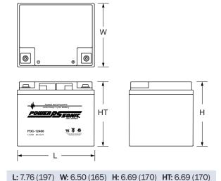
Tolerances are +/- 0.04 in. (+/- 1mm) and +/- 0.08 in. (+/- 2mm) for height dimensions. All data subject to change without notice.
