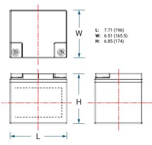
Tolerances are +/- 0.04 in. (+/- 1mm) and +/- 0.08 in. (+/- 2mm) for height dimensions. All data subject to change without notice.
