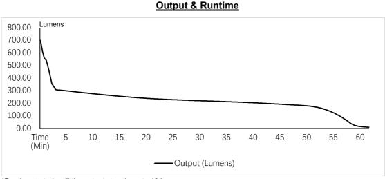
\*Runtime tested until the output step down to 10 lumens.
